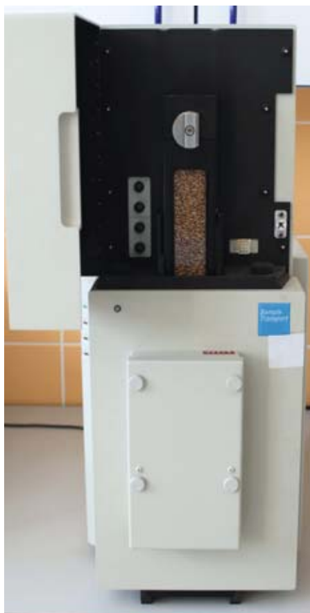
Picture 2: Measuring the intact grain using NIR spectrometry
